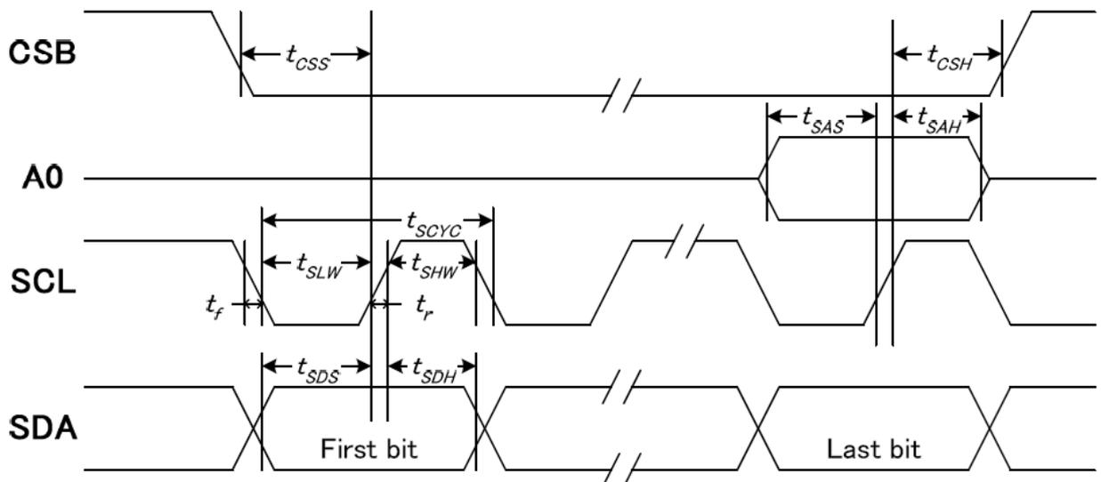
图 3. 从 CPU 写到 ST7567 (Writing Data from CPU to ST7567)
